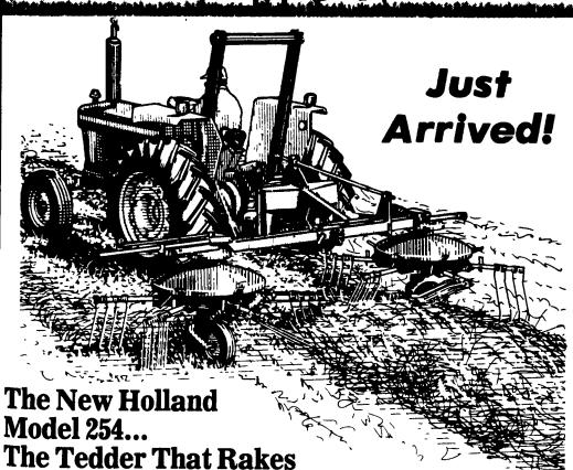
Now you can rake and ted with the same machine — the Model 254 rake tedder. The Model 254 lets you perform a variety of hay-making functions. You can rake a swath into a windrow, rake 2 windrows into one, turn windrows, and move crop away from treelines and fences. And, without tools, you can convert the "254" into a tedder that fluffs up wet, matted-down crop for quick drying. Stop in and let us show you the flexibility of the Model 254 rake tedder.
