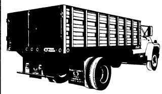
Omaha Standard's solid steel stake sides are designed for confined cargo or bulk hauling, and are ideal for landscapers, trash haulers and contractors. They fit both our Standard and Metro platforms and come in heights of 28", 40" and 52". These sides are available with the standard solid front or an optional steel bulkhead with full width mesh window.
