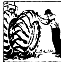
After driving your tractor for up to 1000 ft. if your dual wheel alignment is needed.
