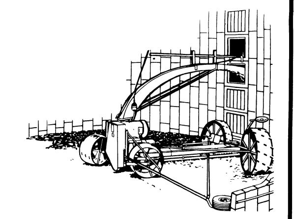
4 Self leveling device provides uniform silage removal 5 Raising hitch (optional) can be permanently mounted
