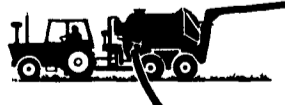
Using 6" side valve and hose for pumping out open pits or under building
