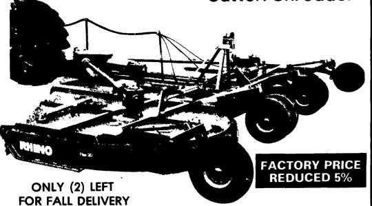
The best 20 foot Cutter made! 540 or 1000 RPM Hyd Fold & Lift Dishpan or Bartype Blade Carriers, Equal angle Driveline Shielded 45R/55R Drivelines Power Divider Gearbox Three Torque Limiters Self-leveling Tongue and Clevis Gearbox Shields, Chain Guards standard
