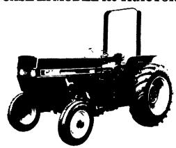
• 42 PTO H.P. • Snychromesh 8F/4R Diesel Transmission Tag #UT1497
