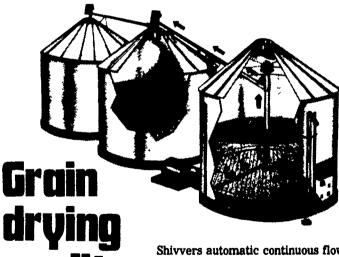
Shivvers automatic continuous flow grain drying systems eliminate the over-drying often caused by slow stirring devices. The Shivvers' secret is the tapered sweep
