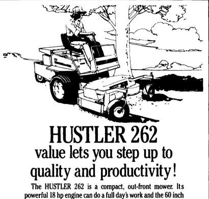
3-way deck, combined with HUSTLER maneuverability, means high productivity, too. The agile 262 has all the "HUSTLER Tough," commercial-quality features, including dual-hydrostatic direct-drive, true zero-degree radius turning, and the easy maneuverability of one-hand twin-lever steering. Its optional 16 bushel BAC-VAC<sup>™</sup> makes it easy to do a neat, clean job.
