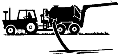
Using 6" side valve and hose for pumping out open pits or under building
