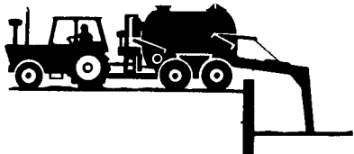
Loading out of open pit with cement sides
