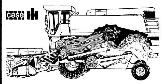
The one moving part in Axial-Flow's entire threshing/separating process is the single large-diameter rotor. Nothing more. No cylinder, beaters or straw walkers. There's far less that can break or need maintenance. That's Axial-Flow combine simplicity.
