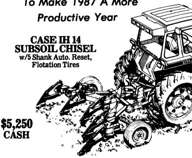
Works behind high horsepower tractors to open soil down to 20" for deep-down penetration of water and air. Parabolic curve shanks lift soil vertically for a wide area of soil fracture. Shank design and V-shape frame combine to deliver easier penetration, reduced draft and less fuel consumption.
