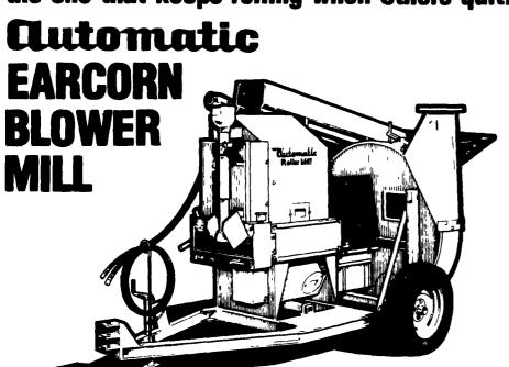
Automatic pioneered the development of the unique crusher unit which shells corn and shreds the cob ahead of the rollers which crack the kernels and reduce the cob further. No troublesome screens to change or slow down the capacity. It comes with 8-foot hydraulic intake auger and 54-inch blower. Also available with an 11-inch tilting discharge auger with 10-foot reach in place of the blower.
