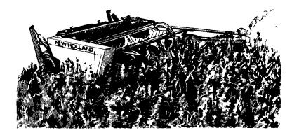
The Model 472 Haybine "mower-conditioner gives you fullwidth conditioning in a seven-foot machine. The torsion bar system on the exclusive chevron rolls lessens pressure to let slugs through. No plugging, less down time
