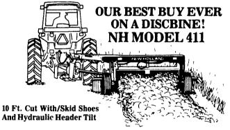
The Model 411 Discbine TM disc mower conditioner keeps on going even in your toughest crops. Six discs make a 10-foot wide cut. They Il mow through fire ant hills and gopher mounds—and slice under down—tangled crops—Seven-foot wide in termeshing rubber rolls condition your crop gently and thoroughly for faster drying You can lay down a wide swath or switch to windrow in seconds without tools
