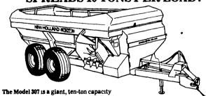
slurry spreader from Sperry New Holland It spreads a fine top dressing of manure - fast! You get an aggressive springloaded auger to move material to the front right side for easy, consistent spreading. The auger floats over rocks and foreign matter, reducing the chance of
