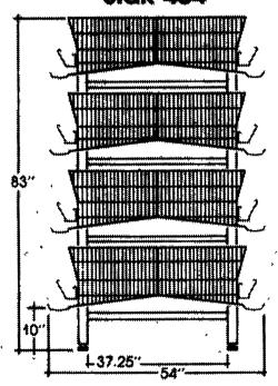
Four tiers, 54-inch width overall, with quiet running bett manure removal. Cages installed in 8-toot sections. Cage size options: 12"x20"; 16"x20" and 24"x20"
