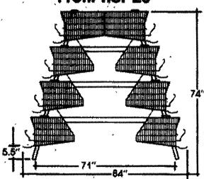
Four tiers of low profile, 20" deep cages on a condensed row width for very high capacity without crowding. Available in 8-foot or 10-foot sections. Cage size options: 12"x20": 15"x20"; 16"x20" and 24"x20",
