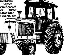
MODEL 4050 100 HP 466 Cu. In. w/4 Post Roll-Gard, Power Shift Trans., Dual Remotes, 18.4x38 Radial Tires, Engine Coolant **Heater & Front Weights**
