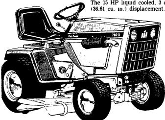
The 15 HP liquid cooled, 3 cylinder Diesel engine has a  $600\ \mathrm{cc}$ (36.61 cu. in.) displacement. 64 mm Bore with 62.2 mm stroke
