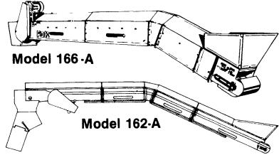
Built rugged for efficient, high-volume feed handling. Economical chain-and-flite action moves feed smoothly without sifting or separating.
