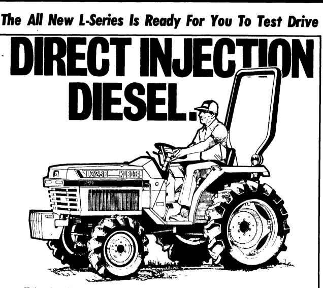
Kubota introduces a compact tractor with direct fuel injection. The new L2250 has a 3-cylinder diesel engine with 21 PTO horsepower. Plus it has direct injection for improved starts in cold weather and better fuel economy, too.
