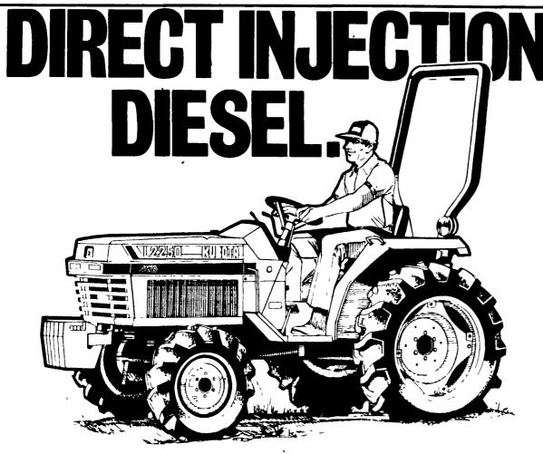
Kubota introduces a compact tractor with direct fuel injection. The new L2250 has a 3-cylinder diesel engine with 21 PTO horsepower, Plus it has direct injection for improved starts in cold weather and better fuel economy, too.
