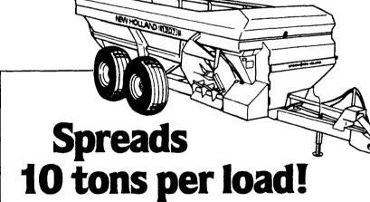
The Model 307 is a giant, ten-ton capacity slurry spreader from Sperry New Holland. It spreads a fine top dressing of manure fast! You get an aggressive spring-loaded auger to move material to the front right side for easy, consistent spreading. The auger floats over rocks and foreign matter, reducing the chance of damage. And, the "307" is backed by our excellent service and parts program. See one today!
