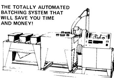
The Computa-Batch is an on-farm feed processing system that will automatically select, weigh, grind, and mix up to 12 ingredients with 99 9% accuracy. Based on tests in actual feeding sit uations, the Computa-Batch will save 15 to 50% in costs over a PTO mixer/grinder or buying finished feed. Ask for a FREE COST COMPARISON ANALYSIS to see how much your actual savings would be
