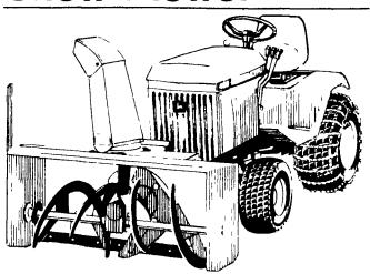
New two-stage snow blower for heavy snow conditions Features 16-inch impeller clears a 47 in swath. Adjustable skid shoes spout deflector hydraulic chute angling and drift blade
