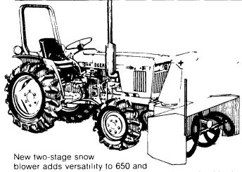
750 Tractors Front-mounted attachment has a durable drive system Features shear-bolt protection adjustable spout deflector and skid shoes hydraulic chute angling and lift control and drift knife. Cuts a wide 59-in swath.
