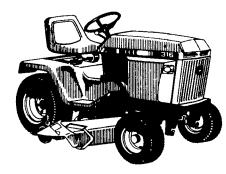
The 16-hp 316 and 18-hp 318 have hydrostatic drive, hydraulic lift and heavy-duty engines Built-in headlights high-back seat and color-coded controls are also standard Mower, thatcher, front blade, tiller, snow thrower, material collection systems available
