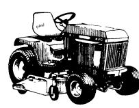
Rugged Reliable The 20-hp 420 has 2cylinder gas engine The new 20-hp 430 has 3-cylinder diesel engine Both have heavy-duty drivetrains, differential lock Plus power steering, 26-inch turning radius, hydrostatic drive and hydraulic lift
