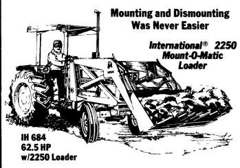
2250 Mount-O-Matic has a 101/2-foot dump and is ideal for 40 to 80 horsepower tractors.
