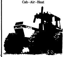
MFD (Mechanical Front drive) for Case 2094 and 2294 tractors offers you the fuel-saving, weather-beating productivity boost of four wheels pulling with limited-slip differentials MFD plus new 12-speed power shift and new electrically actuated differential lock work together to create Case over-100-horsepower units of impressive working ability
