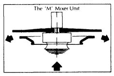
The FRISTAVENT uses a CENTRIFUGAL fan that lays out a continuous CARPET of air, this ensures an EVEN DIS-TRIBUTION OF FRESH AIR to the livestock with NO DOWN DRAFTS.
