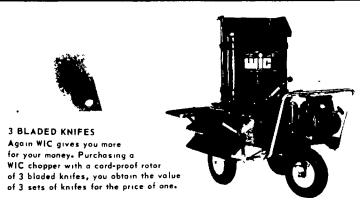
GONE FOR GOOD, THE EXHAUSTING JOB OF CHANGING THE KNIVES, AS THE 144 BOLTS AND NUTS HAVE BEEN REPLACED BY 8 RODS INSERTED THROUGH THE KNIVES WHICH ARE COLLECTIVELY TIGHTENED, FORMING A ONE PIECE ROTOR.
