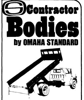
Rugged, all-steel 14 sides and 96 wide platforms Available with 28, 40 and 52 high heavy duty steel bulkheads with full width steel mesh windows Standard three-way express tailgate or optional double-acting tailgate with forward controls Swaged (indented) 3-light cluster in rear outrail for better light protection and appearance. These tough fieldproven units, teamed with job-matched Omaha Standard pists are total working units superior to any on the market
