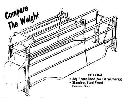
This European style Farmer Boy crate reduces creep crushing because it is narrow at the top and wide at the bottom. This design prevents the sow from turning and ensures that she takes extra care in rising and lying down. The front and back doors open easily and without losing pins, with the new style J pin. The all welded construction, hot-dipped galvanized after fabrication, eliminates sharp edges that can cause injury.
