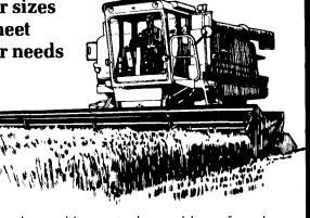
They re the world's most advanced line of combines Because a rotor replaces the conventional cylinder and troublesome straw walkers. Threshing and separating are more thorough — there are fewer cracked kernels. and there is less downtime and fewer repairs
