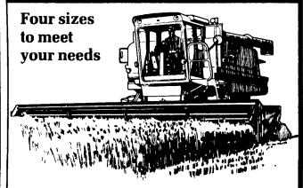
They re the world's most advanced line of combines Because a rotor replaces the conventional cylinder and troublesome straw walkers. Threshing and separating are more thorough—there are fewer cracked kernels and there is less downtime and fewer repairs.
