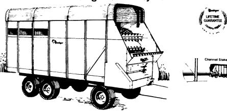
A Badger Box is built with steel channel side stakes for extra strength and specially treated, exterior grade plywood to resist acids, corrosion, and rot. The bolted undercarriage and chain drive are designed to take the toughest punishment.
