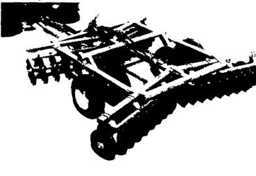
The MF 233 pull-type tandem disk harrow is available in 7'8" to 12'4" cutting widths, and is well suited for small to medium acreage applications.
