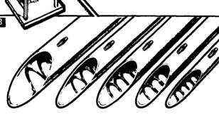
Chore-Time's genuine FLEX-AUGER' IS available in 5 models, with capacities ranging from 15#/min. to 220#/min. Two systems also available for High Moisture Corn.
