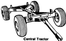
Wagon Gears eaturing one piece steering rod, all-welded construction, rear hitch, and pressure type grease fittings. Bolster stakes can be set at 38 ' or 42" width Gear capacities are gross weight at farm tractor speeds. All units comes
