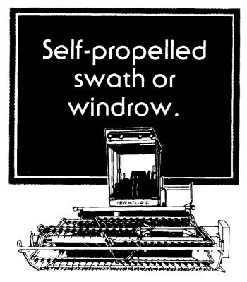
YOU CAN'T BEAT A SELF PROPELLED FOR CONVENIENCE AND COMFORT. THE FORD GAS OR PERKINS DIESEL DOES ALL THE WORK FOR YOU. THE ROLAREEL HEADER' GENTLY SWEEPS THE HAY INTO THE WIDE 110" CHEVRON INTERMESHING RUBBER ROLLS
