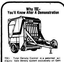
TDC. Total Density Control is a patented airdraulic bale density system exclusively on Gehl round balers. This remarkably simple system allows you to vary bale density and core size to adapt to changing crop conditions, giving you the flexibility you need to make quality round bales you libe proud of Both the new 1860 and 1460 feature texturized upper belts lower bale forming rollers. 3 ball twine box and the new optional Auto-Electric Twine-wrap
