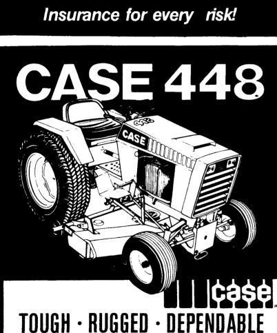
The Case 448 is everything you'd expect...a powerful all-purpose tractor for lawn, yard and garden care. It has an 18-hp Onan twin-cylinder engine with hydraulic drive and attachment lift. Rugged cast iron front axle, heavy-duty king pins and welded steel construction. High clearance frame, with big 16" rear wheels, plus electric start, makes this powerful machine a natural choice for big-job chores.
