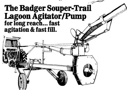
Now you can pump solid or liquid manure from storage basins quickly and efficiently without the need for ramps or
