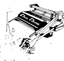
Avco New Idea mower conditioners produce hay that dries fast and evenly. Hay is fluffy, well mixed and cures "ready to bale" in as short or shorter time than that produced by other types of mower conditioners.
