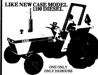
43 HP w/12 Speed Syncro Trans., Hyd. Remote, 13.6x28 Rear Tires, 540 Independent PTO, 3 Pt. Hitch. ALSO IDEAL FOR LOADER PURPOSES! Factory List Price Over \$15,584
