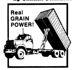
Heavy gauge steel sides with deep corrugations for maximum strength. The stakeless is available with either 52 or 60 high sides and standard lengths of 18 20 22 and 24 Greater inside width and length Ideal for hauling grain sugar beets bagged or palletized products
