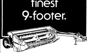
Full width conditioning rolls in the Model 489 Haybine mower conditioner are located in the main frame, not the header. The lighter header responds quicker to ground contours and greatly reduces knife and guard damage. The 489' is designed for operators who demand the very
