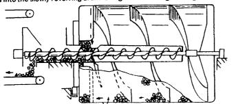
The spiral flights are designed to carry the feed back to the front into the reversed
