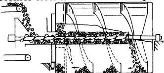
In filling the Roll-A-Mix, feed is carried by the auger to the rear of the mixer where it falls into the slowly revolving drum for a gentle tumbling thorough mix
