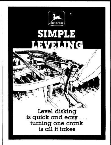
Leave your wrenches in the tractor: drawn Level-Action™ disks have a simple crank adjustment.
