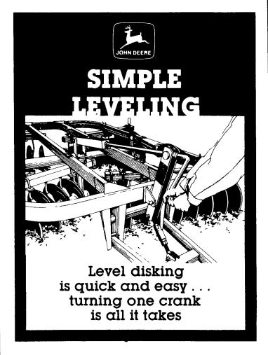
Leave your wrenches in the tractor: drawn Level-Action™ disks have a simple crank adjustment.
