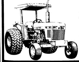
Two brand-new fuel-efficient tractors designed to handle demanding jobs. Both have a 4-cylinder liquid-cooled diesel engine — 55 gross hp 50 PTO hp on the 1450 67 gross hp 60 PTO hp on the 1650 Plus 3-range collar-shift transmission with 9 forward 2 reverse speeds inboard planetary final drives independent live 540-rpm rear PTO opencenter hydraulics Category 2 3-point hitch power steering hydraulic wet-disk brakes Roll-Gard\* ROPS and much more Both are available with front-wheel drive
