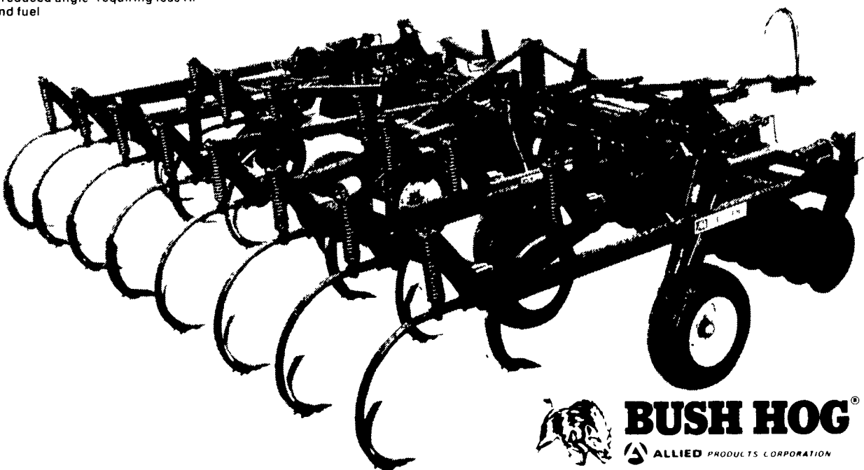
Rigid shanks are recommended for use in soils free of rocks and stumps. Shear pin protection is standard equipment. Shanks contact the soil at a reduced angle, requiring less HP and fuel.
