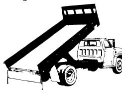
Rugged, all-steel 14" sides and 96" wide platforms. Available with 28", 40" and 52" high heavy duty steel bulkheads with full width steel mesh windows. Standard three-way express tailgate or optional double-acting tailgate with forward controls Swaged (indented) 3-light cluster in rear outrail for better light protection and appearance. These tough, fieldproven units, teamed with job-matched Omaha Standard hoists, are total working units, superior to any on the market
